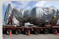
Gas Turbine (371.4 ton)
